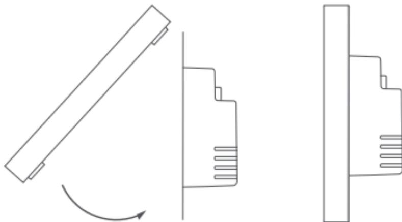
First, tilt the panel downward and align the top portion with the slots.
